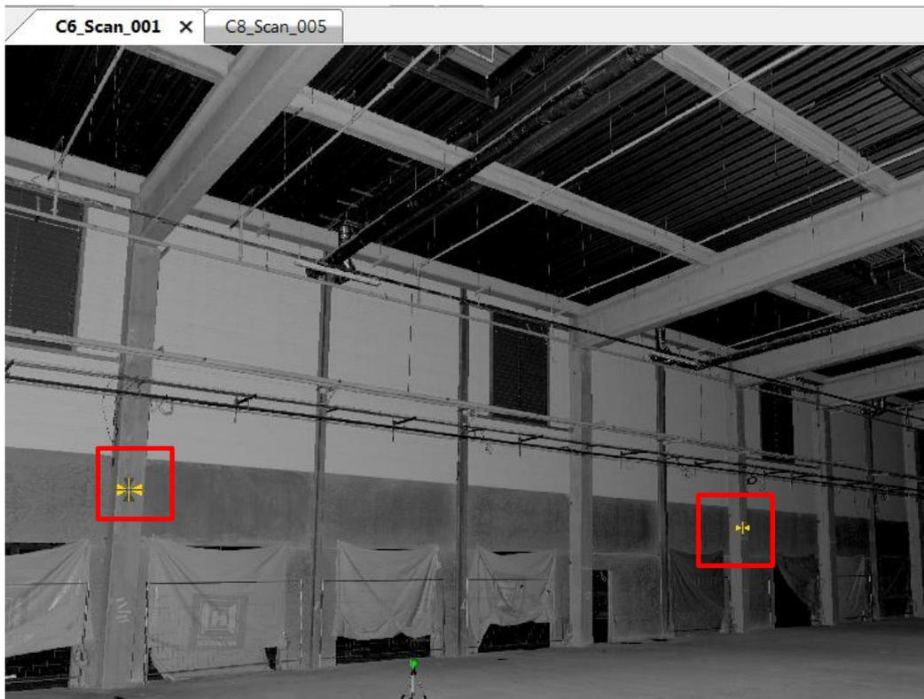
First scan : main wall and columns. Creating of 2 points on the columns front face. These points will be used to orient the scan along the x axis, and also to give a direction for the registration.
