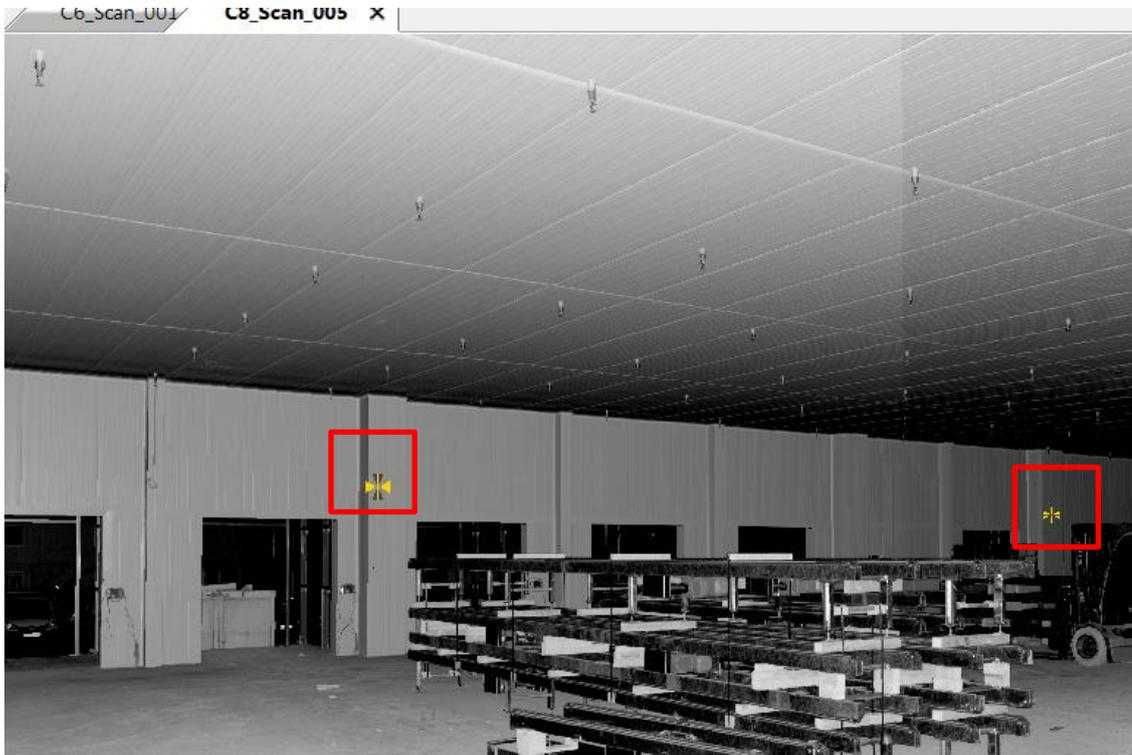
Second scan : the walls and the columns are insulated. But the direction is still the same. So, we create 2 points on the same columns.
